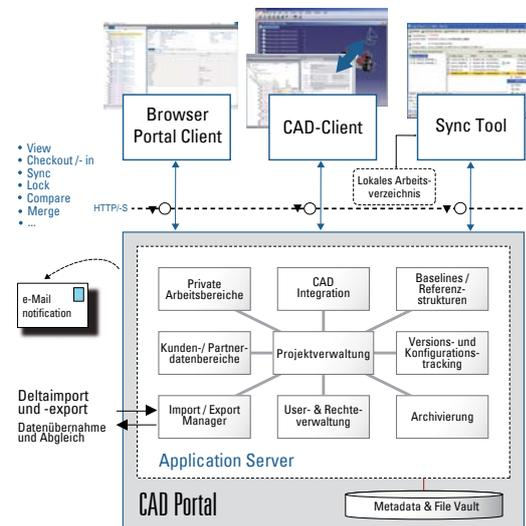
CAD users synchronize local data with the portal's current content. Thanks to a locking mechanism, users cannot inadvertently overwrite other people's data. Changes are made in the CAD client and synchronized with the portal on check-in. When CAD users check in data, they see a transparent overview of the local changes and their impact on the assembly in the portal.
